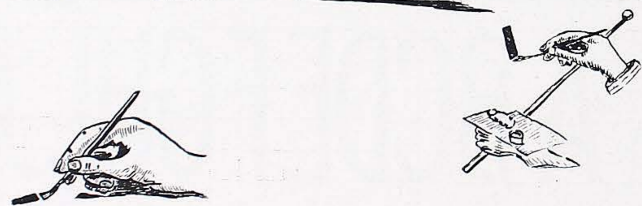
Correct Position for Brush both with and without the Use of Mahl Stick
