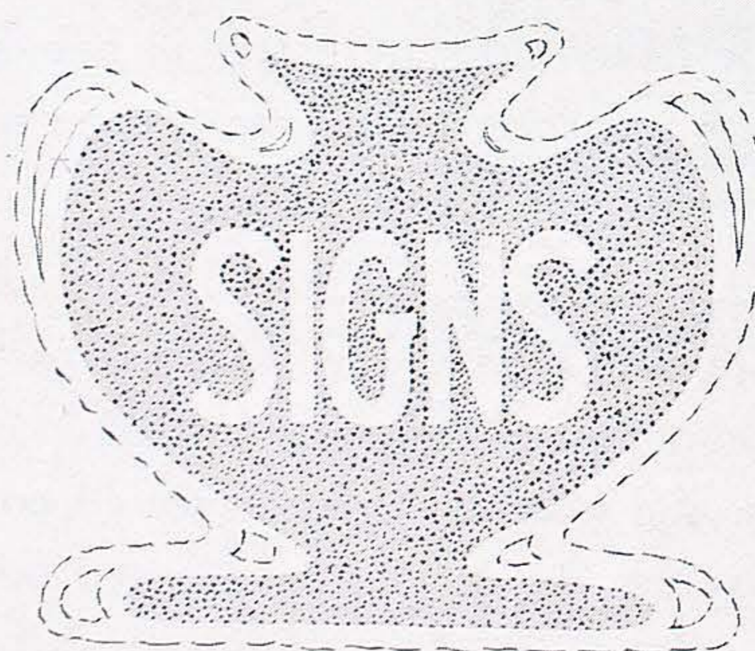
A - EMBOSSED PANELS ON BOARD SIGNS
