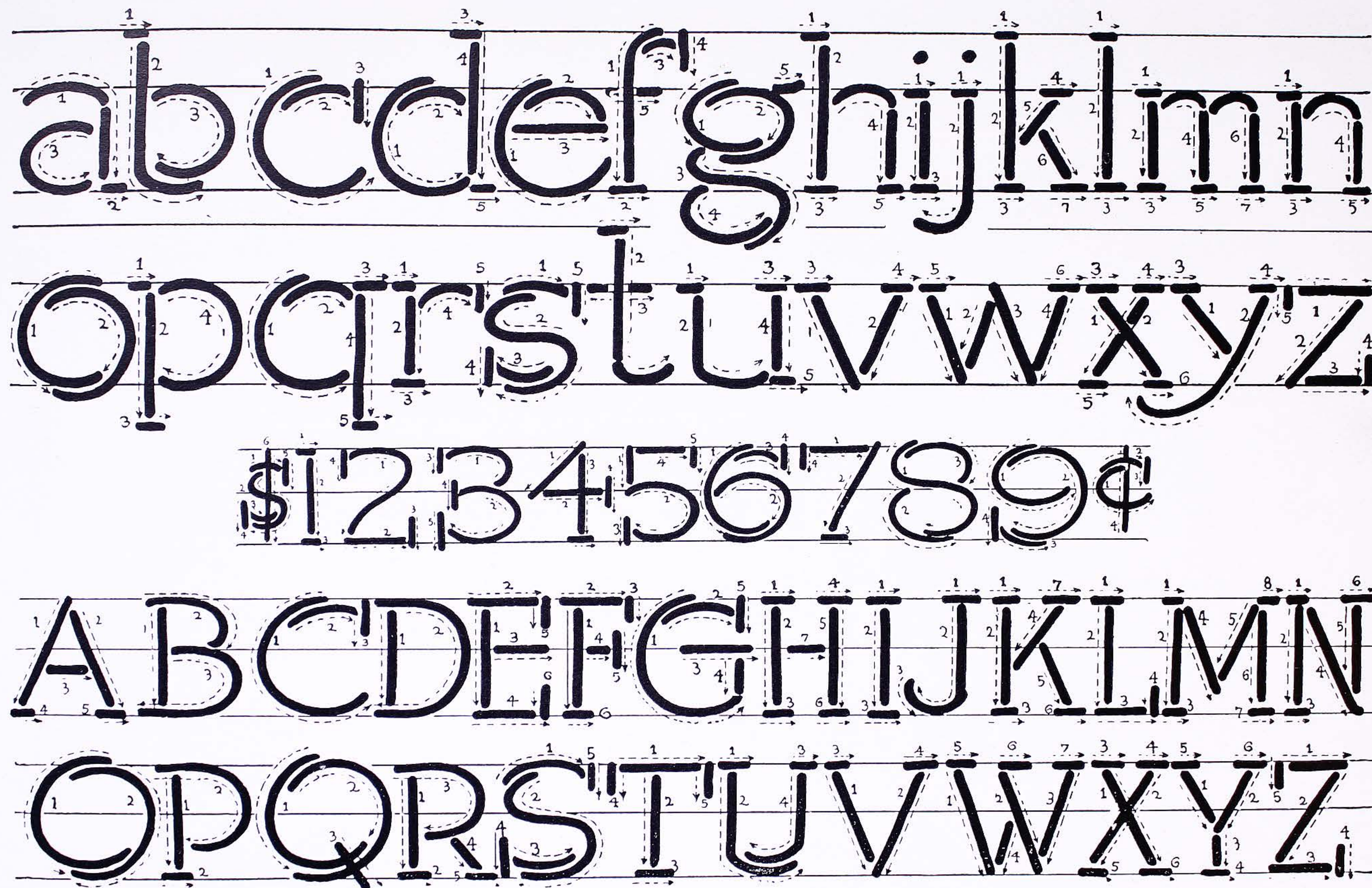
Broken strokes show construction of "Beginner's Alphabet." Numbered arrows indicate the order and direction of elements. Made with Style B Speedball.
