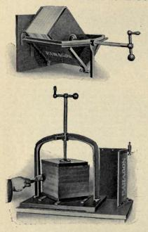
This press is made wholly of iron, excepting the adjustable squaring-boards, and consequently will not twist or warp under pressure, thus throwing the adjusted paper out of line.
