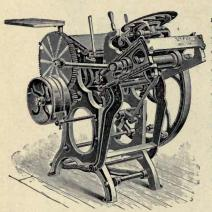
This press runs easily and quietly and is so well balanced that its speed is limited only by the ability of the feeder. The distribution is unequaled. The horizontal platen, with long rest, insures speed, ease and accuracy in feeding. Each press is fitted with throw-off, depressible grippers and instantaneous chase clamp, three chases, one brayer, two wrenches, two sets roller stocks and one roller mould. If desired two extra chases or three cast rollers furnished instead of the mould.
