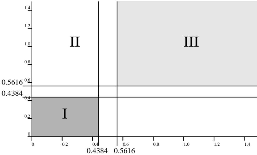
**Fig. 4.** The complexity regions: in I, the output size dominates. In II, the 1-d complexity term is largest, and III is like point search
