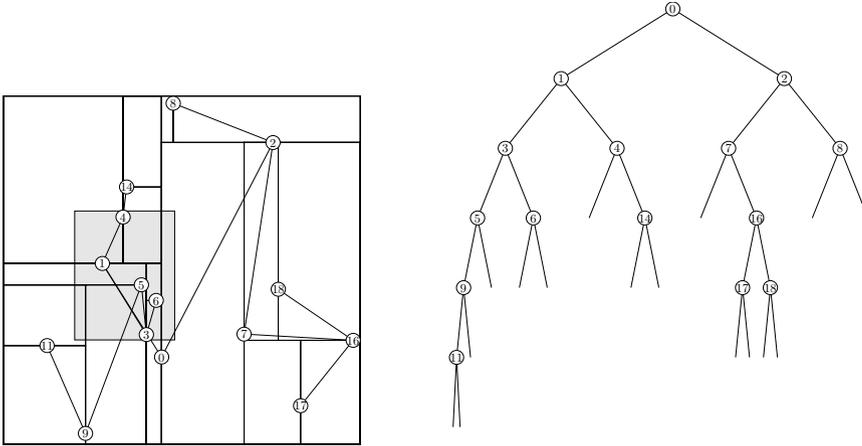
**Fig. 1.** The k-d tree and its partition of the plane. The query rectangle is shaded
