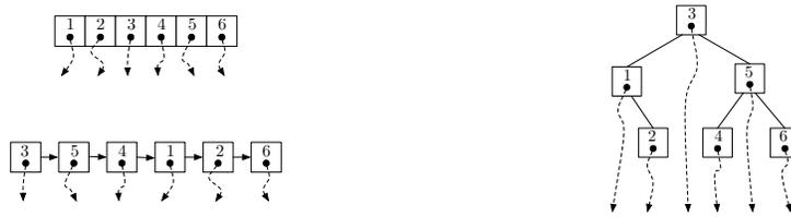
**Fig. 2:** The different node structures used for the standard (top-left), list (bottom-left) and bst-trie (right) when the order of appearance of the characters is 3, 5, 4, 1, 2 and 6. The dashed arrows represent the pointers to further levels of the trie.
