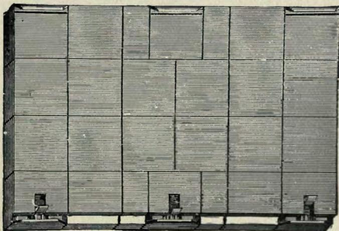
The cut shows a page of the sectional blocks, with the hooks and catches, ready for the plate. The hooks are operated by a ratchet, the same as those on the patent wood blocks. The sections are made in the following sizes: 1×4, 2×4, 4×4, 1×8, 2×8, 4×8, and 8×8 ems pica. In five minutes a page can be made up to fit a plate of any size.
