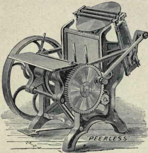
The strain-bearing parts are of wrought iron or steel, and much heavier than the corresponding sizes of other machines. This insures solidity and an immense strength, and necessary means for creating a powerful impression and resisting a heavy strain.
