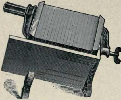
For straightening up and holding sheets of paper while being glued for tablets. Will hold any quantity up to three thousand sheets of paper, and any size from  $2\frac{1}{2} \times 2\frac{1}{2}$  to  $8\frac{1}{2} \times 14$  inches. With an additional clamp and larger press boards almost any size of work can be easily handled.
