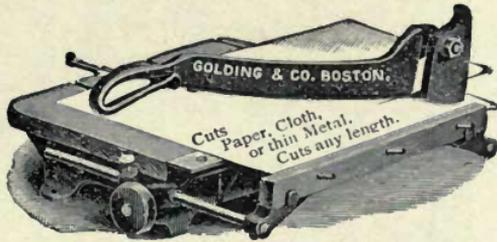
These machines are made in a thorough manner. The frame is of iron and the table of hardwood. The front gauge is positive, easily set and accurate, being controlled by a rack and pinion which holds the gauge exactly parallel with the knife. It has a reversible iron back gauge extending 28 inches from the knife, and a side gauge which may be placed in three different positions on the table, according to the size of work being cut.
