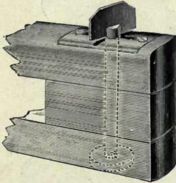
These Files are made of cherry, nicely finished in oil. The fastenings are brass, with steel thumb-screw, having polished heads. The manner of opening and closing the File to insert a sheet is quite novel and simple. The clasp end of the File has a flat headed thumb-screw which is passed through a slot, and by giving screw one quarter turn the File is securely locked.
