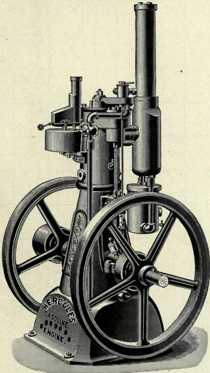
The Hercules is the latest gas and gasoline engine in the market, and embodies all recent improvements. It is built in three styles: single, vertical; double vertical; and horizontal. The charge is ignited by a glowing tube. No battery is required, and the charge never fails of ignition. It is the simplest, most powerful and reliable, and consequently the cheapest gasoline engine in the market.
